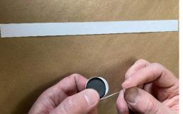
Start by rolling one of the .75"x11" strips of paper around the three magnets as shown in the photo to make a paper tube.
